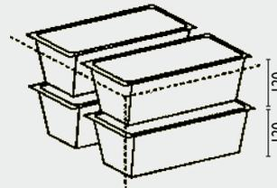
**2 static pack evaporators (with defrosting heater) + evaporator coil foamed in the walls**
